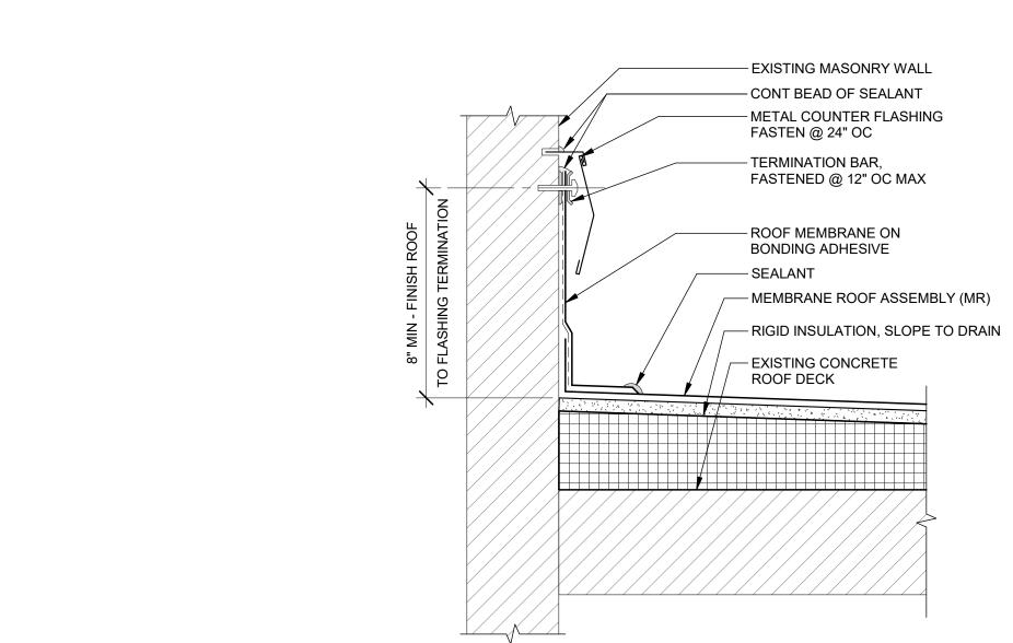
FLASHING AT BEARING WALL
