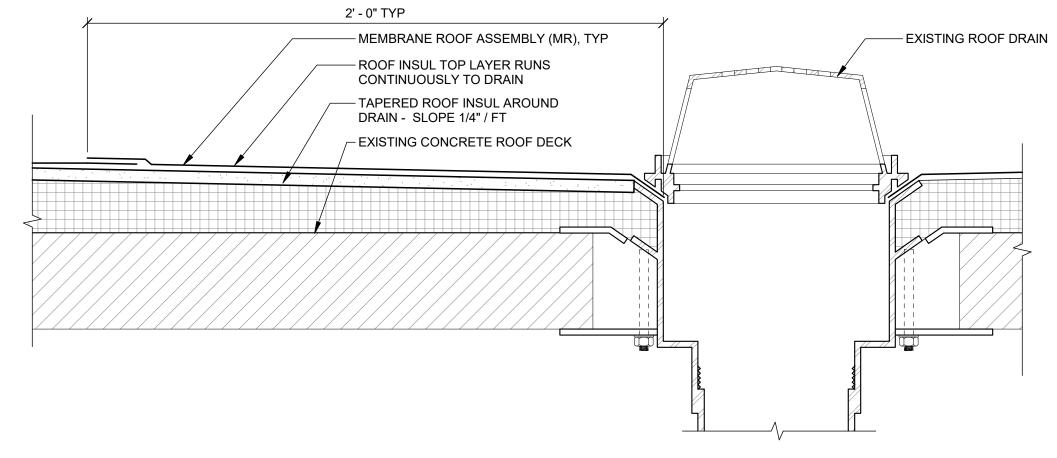
ROOF DRAIN - FLAT CONCRETE SLAB
