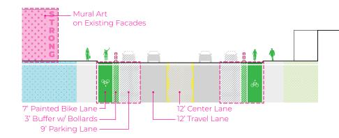
In the short term, update the configuration of Warren street. Use high-visibility paint and flexible bollards to establish designated bike lanes and protected buffer zones. The parking lanes will create further separation between cyclists and drivers, while maintaining the amount of available parking. Additionally, collaborate with existing businesses and pursue funding for mural art on existing facades to create a more hospitable and inviting streetscape.
