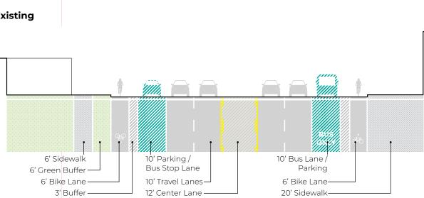
Currently, Livernois has two, one-way bike lanes on both sides of the street, which are separated from traffic by a 3' buffer lane and hybrid bus stop/parking lanes. However, the bike lanes are unpainted, and with a 90' total width, the street is difficult to cross for bikers and pedestrians.
