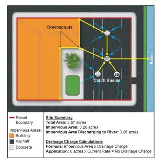
Figure 2: 100% Stormwater Discharge to Surface Water
