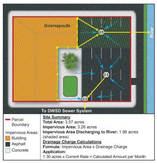
Figure 3: Partial Stormwater Discharge to Surface Water
