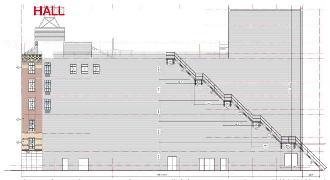
West elevation drawing showing approved (not yet installed) fire escape. Image from HDC2024-00066 application documents. Note that this image does not depict the existing fire escape as that proposal initially included removal of the existing fire escape; that aspect of the proposal was later withdrawn.
