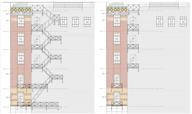
Left: Elevation showing existing conditions. Right: Elevation showing proposed work. Images from application documents.
