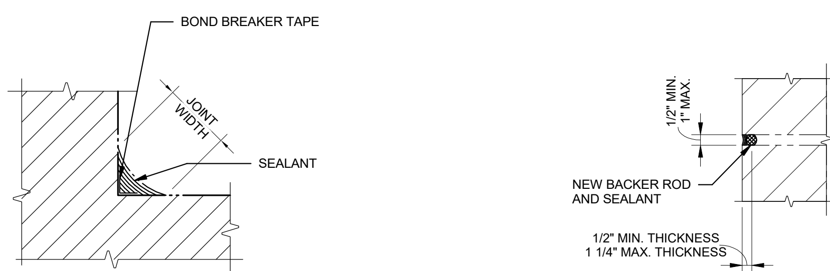
D3 TYP. - COVE SEALANT JOINT SCALE: 3" = 1'-0"
