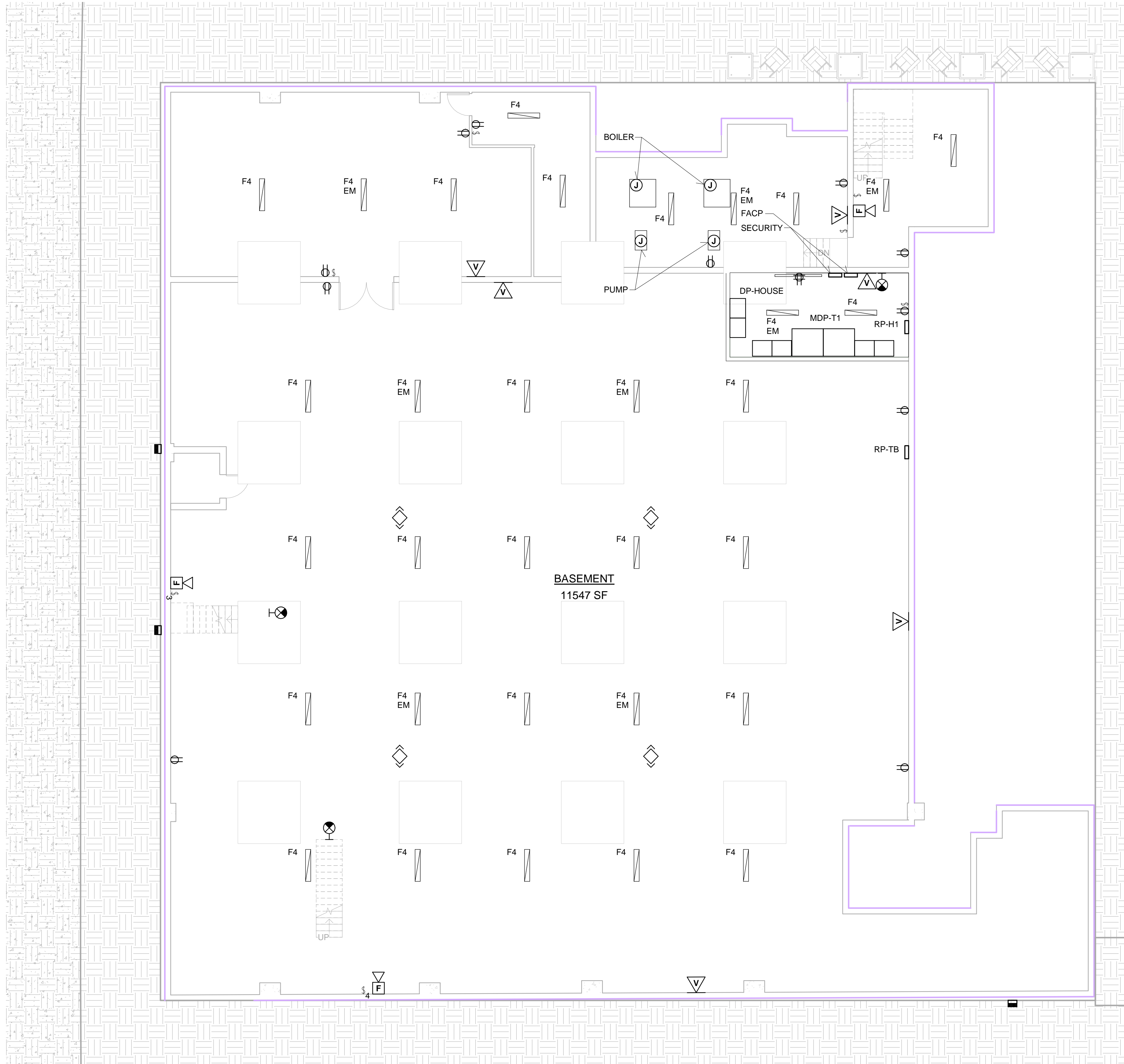
① BASEMENT ELECTRICAL PLAN 1/8" = 1'-0"
