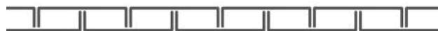
Mid-point to mid-point: minimizes the appearance of the flanges, creates an attractive tightly ribbed visual profile
