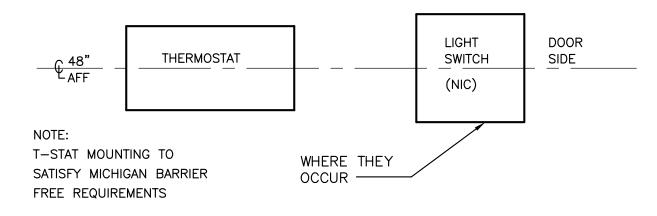
TYPICAL THERMOSTAT MOUNTING DETAIL
