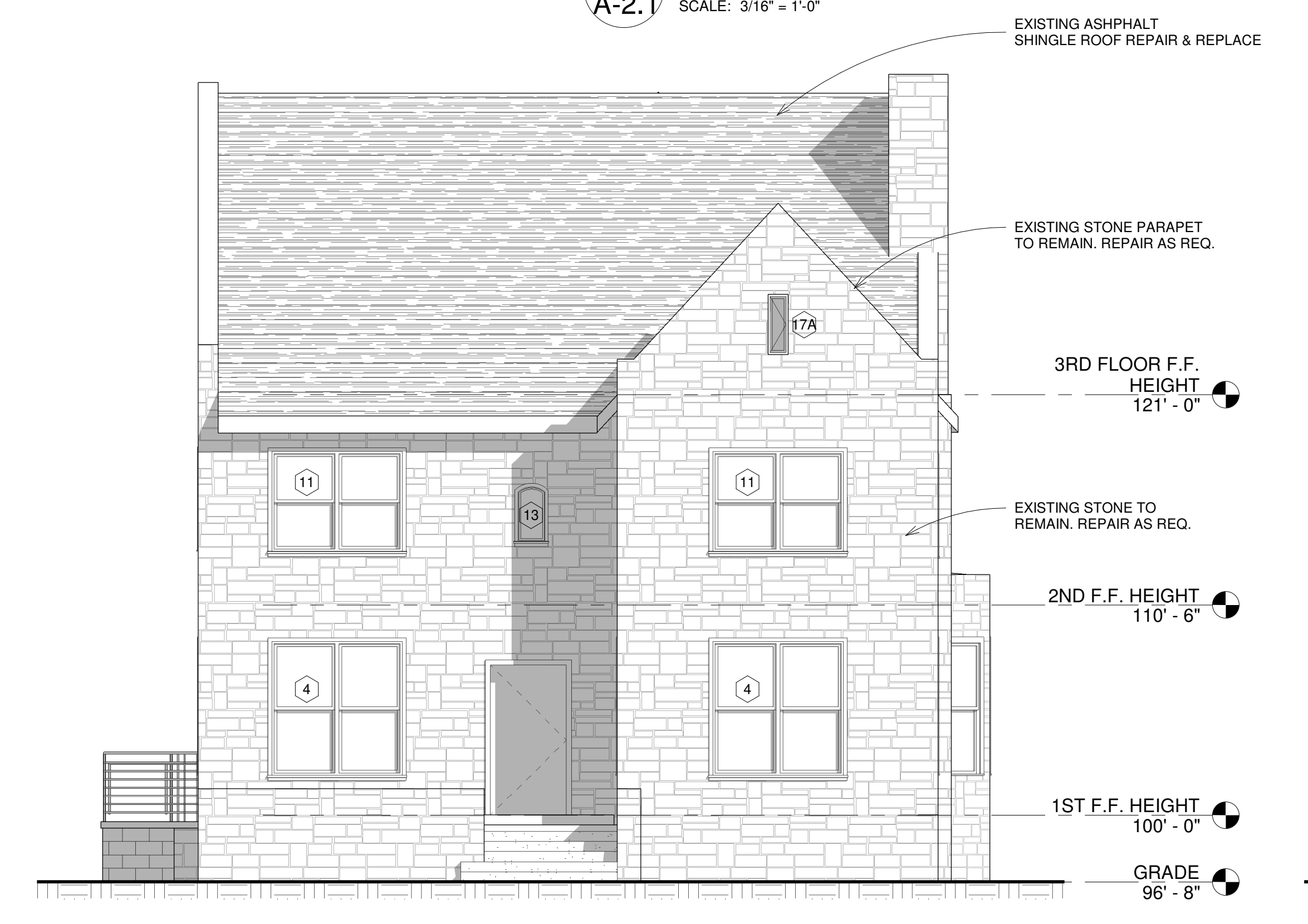
3 SOUTH ELEVATION A-2.1 SCALE: 3/16" = 1'-0"
