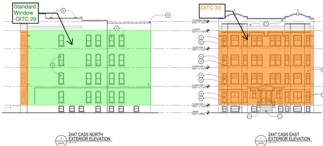
Figure 6: 2447 Cass Street- Window upgrades North and East Facades
