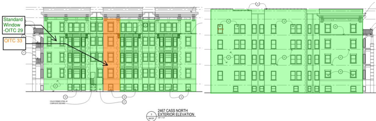
Figure 4: 2467 Cass Street- Window upgrades North and South Facades
