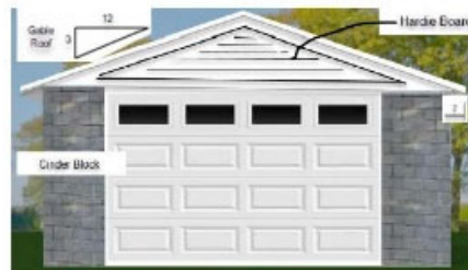
Front Garage Elevation
